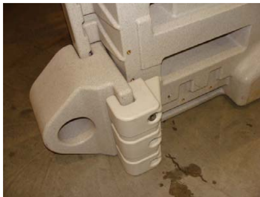
C-clamp bolted into place at Port front
