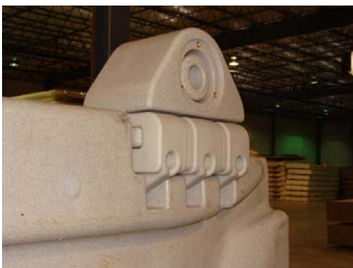
Post attachment bolted into place at the side rear position
