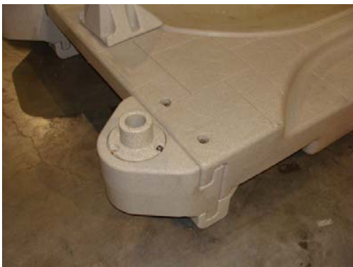
Pipe Adapter bolted in place
