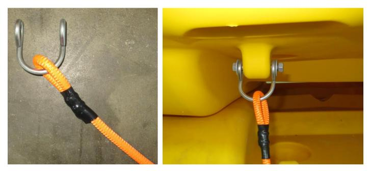
4. Repeat the process above to attach the bungee cord to the second connection point. Attach a rope, chain or cable to the bungee clip and run this down to the anchor. The bungee cord should be slack so it has minimal tension on it. Repeat on other end to complete the installation.
