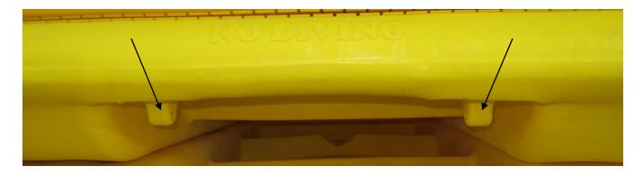
3. Insert one of the u-shaped clevises through the loop in the end of the bungee cord. Place the clevis over the attachment point on the raft. Insert the 7/16" bolt and washer through opening and secure with the 7/16" tri-lock nut and washer. The nut is a locking nut and will require a slight amount of force to thread on.
