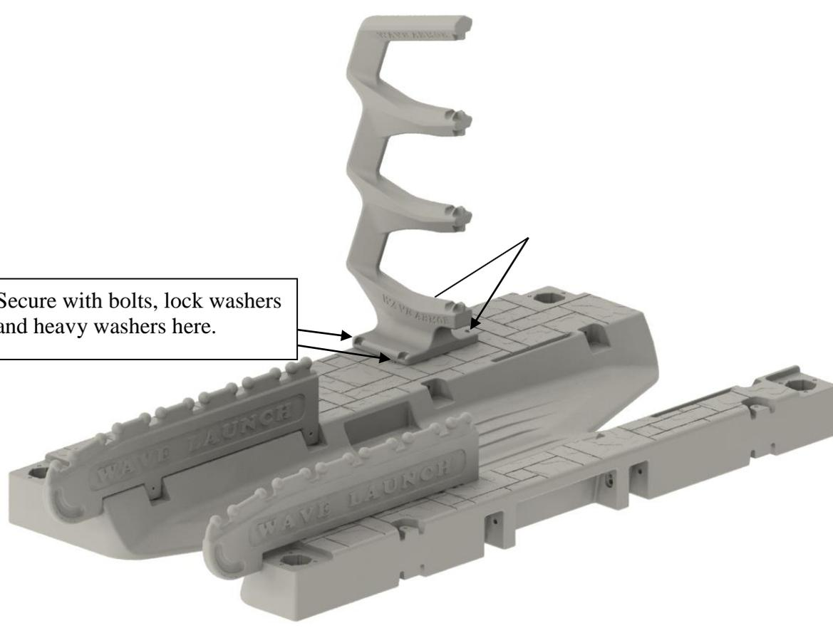
Secure with bolts, lock washers and heavy washers here.
