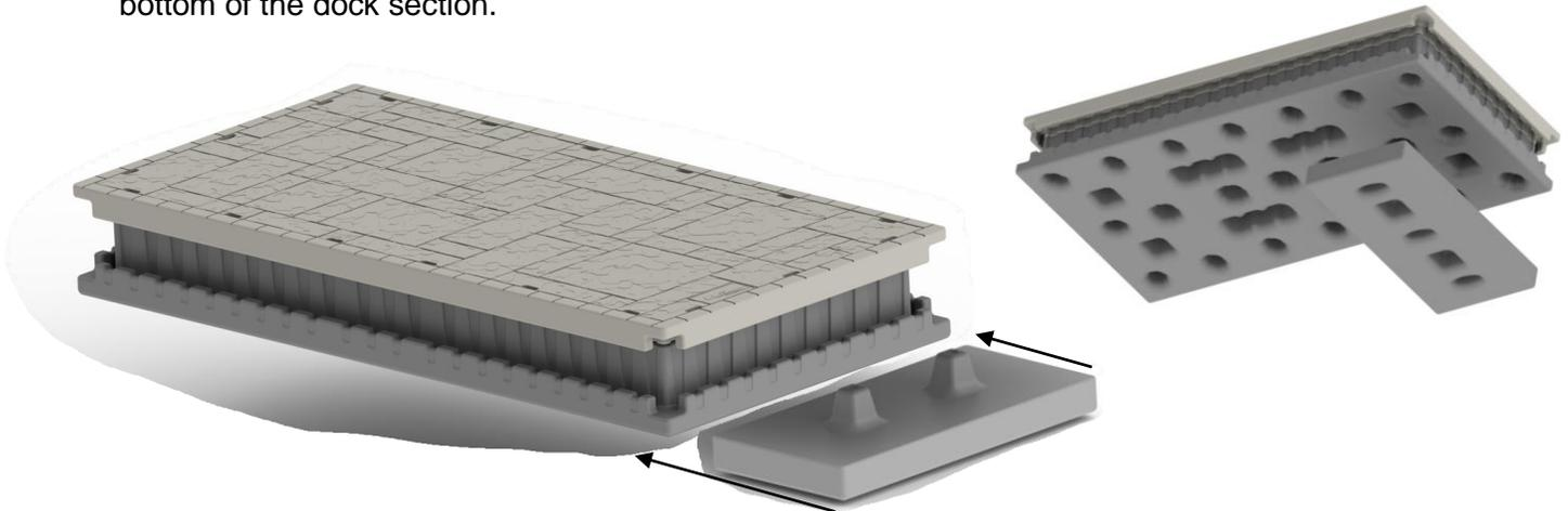
2. Push the booster under the water and under the dock section until the tabs lock into the dock. **Caution: Keep hands and fingers clear so they are not trapped between the booster and the dock section.**
