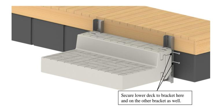
**3.** Move the lower deck into position against the floating dock. Attach each bracket securely in at least four places using the necessary hardware (not supplied). Completed installation shown below.
