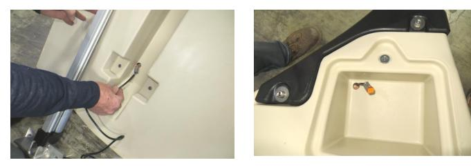
**4.** Bolt the actuator in place using the  $3/8 \times 1$ " bolts, lock washers and flat washers.
