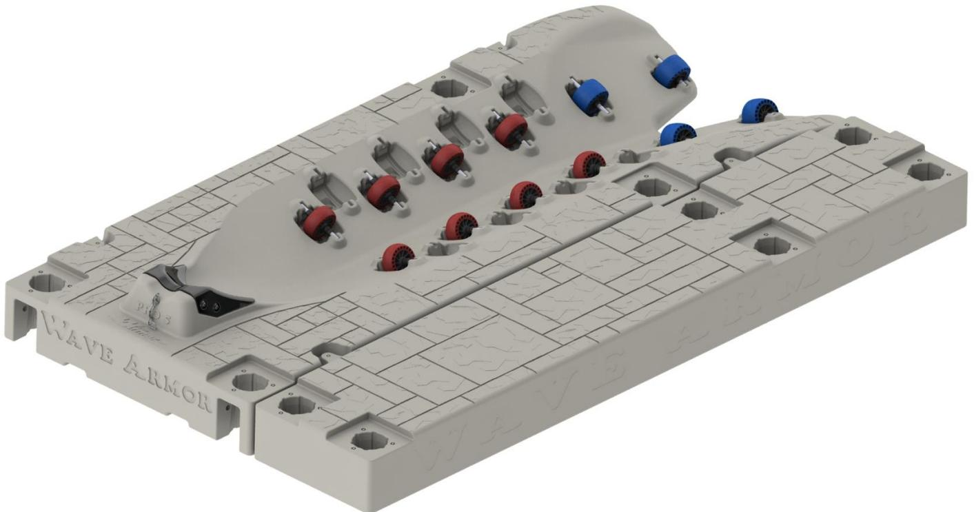
2. Insert the bottom connectors and the top connectors into the post holes and secure with the 3/8 x 1 3/4" bolts, lock washers and heavy washers.
