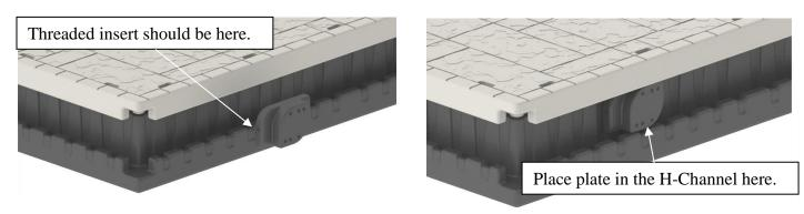
2. Turn accessory plate **clockwise** to lock it into the H-channel on the dock. It can usually be turned by hand but two bolts may be threaded into the face to make it easier to turn. Slide plate in the channel to align the threaded insert with the slot in the dock deck.
