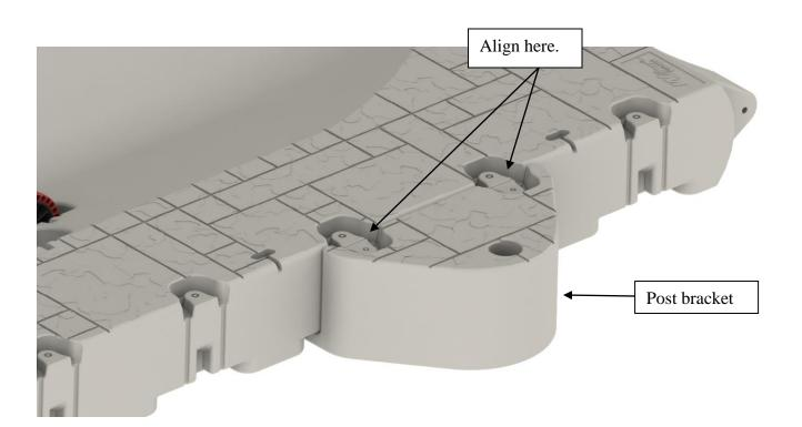
2. Install cap connectors into the recessed areas on the bracket and the port. Secure with the 1  $\frac{1}{2}$ " bolts, lock washers and heavy washers.
