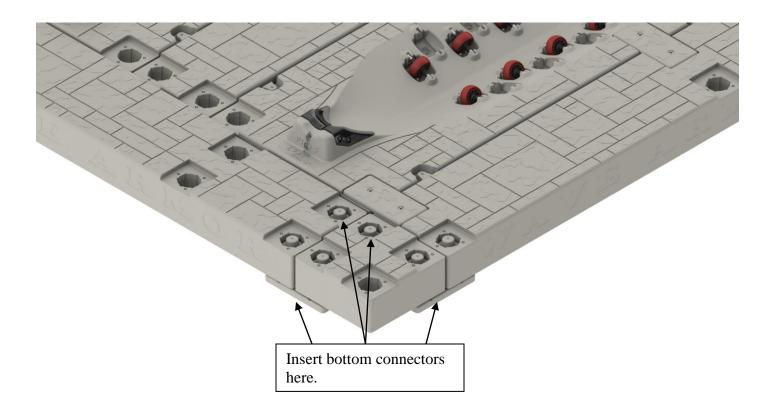
**3.** Secure the corner section to both the side and front extension decks with the 3/8 x 1 ¾" bolts, lock washers and heavy washers. Repeat the process on the other end of the front deck extension to complete the attachment. Each corner section and side/front extension are sold separately.
