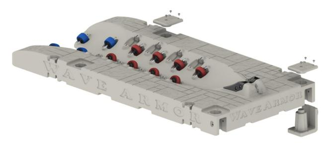
3. Move the port into position alongside the dock. Plastic connectors on the port should align with the connections on the dock. Adjust as necessary. Secure with the  $\frac{1}{2}$  x 9" bolts, washers and nylock nuts.
