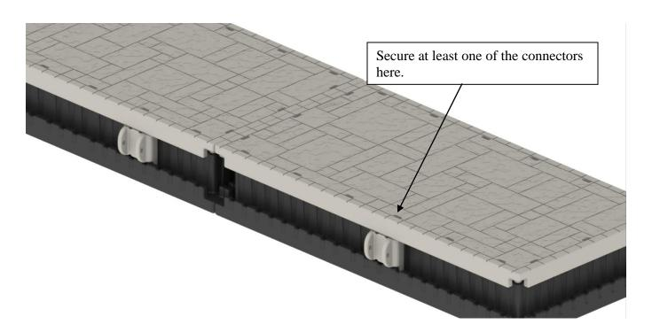
**2.** Attach the plastic side connectors to the port as shown below. Secure with the  $3/8 \times 2$ " bolts, lock washers and heavy washers.
