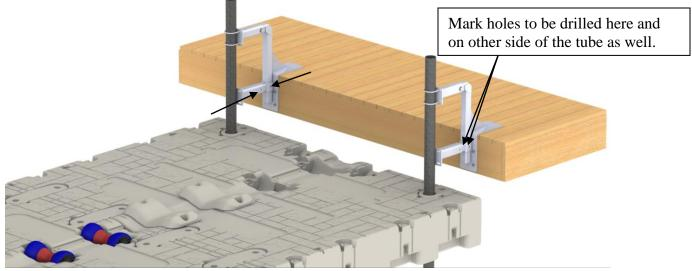
2. Secure tube with the flat plate to the tube with the U-shaped bracket using the ½" x 4" bolt, washers and nut. Insert assembled support tubes into place between the post and the raised mount. Secure to the raised mount using the ½" x 4" bolt, washers and nut.
