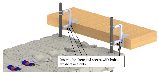
**3.** Attach U-bolts ever pipes and into slots on the flat plate as shown below. Tighten a washer and nut onto each leg of the U-bolt. Once they are tight, thread a second nut onto each leg and then tighten the nuts against each other. This will help keep the nuts and U-bolts from coming loose.
