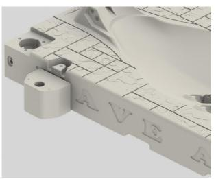
2. Align post attachment top piece with the recessed area on the top of the port as shown below. Place into the recessed area. Secure with 3/8" bolts, lock washers, and heavy washers. Repeat process for second post attachment.
