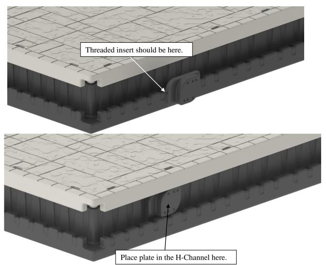
2. Turn accessory plate clockwise to lock it into the H-channel on the dock. It can usually be turned by hand but two bolts may be threaded into the face to make it easier to turn. Slide plate in the channel to align the threaded insert with the slot in the dock deck. Secure with the 3/8 x 2" bolt, lock washer and heavy washer. Repeat process for the second plate.
