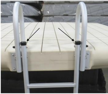
3. Install top right hoop into the raft and secure with the  $3/8 \times 3/4$  bolts using the 7/32" allen wrench. Repeat process for the top left hoop.
